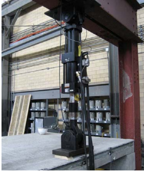
Figure 4.15: MTS Actuator and Load Plate for Positive Moment Specimens
