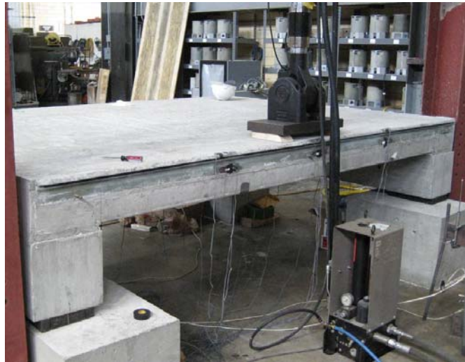
Figure 4.8: Specimen POP1 Before Testing
