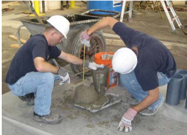
Figure 4.6: Slump Test for specimen POP1
