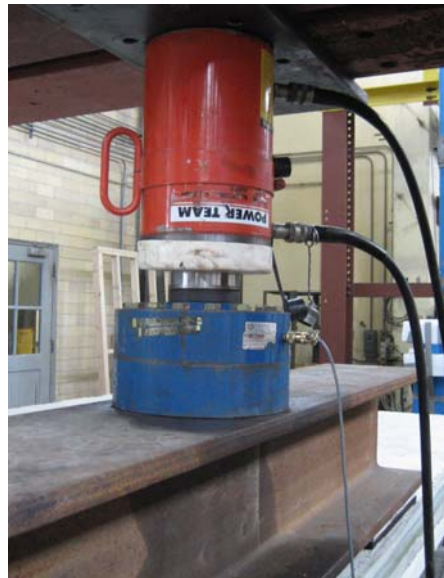
Figure 4.17: Hydraulic Ram Setup Used to Test Specimen NOP2 to Failure
