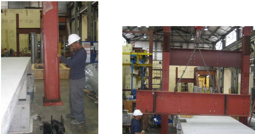
Figure 4.14: Assembling the Reaction Frame for Specimen NOP1
