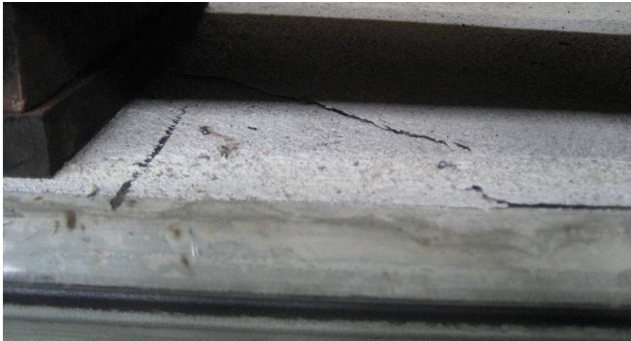
(a) Top of Specimen Near Bearing Pad along NW side of Specimen
