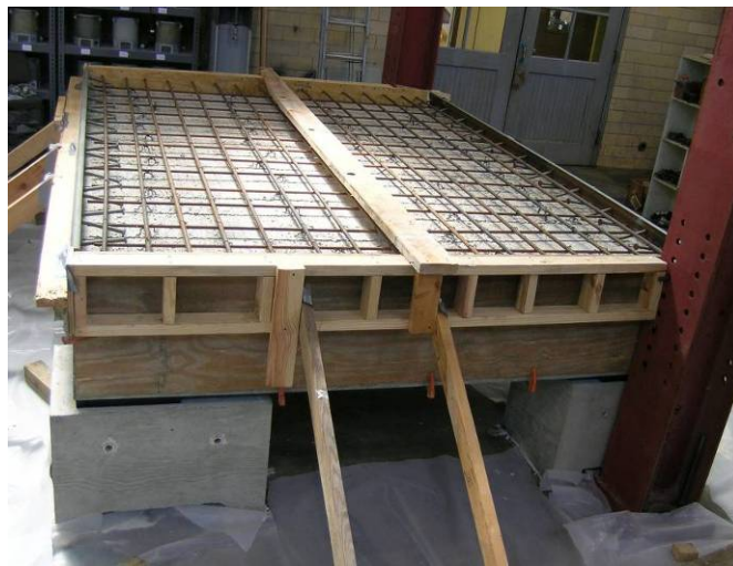
Figure 4.5: Specimen P0P1 Prior to Casting
