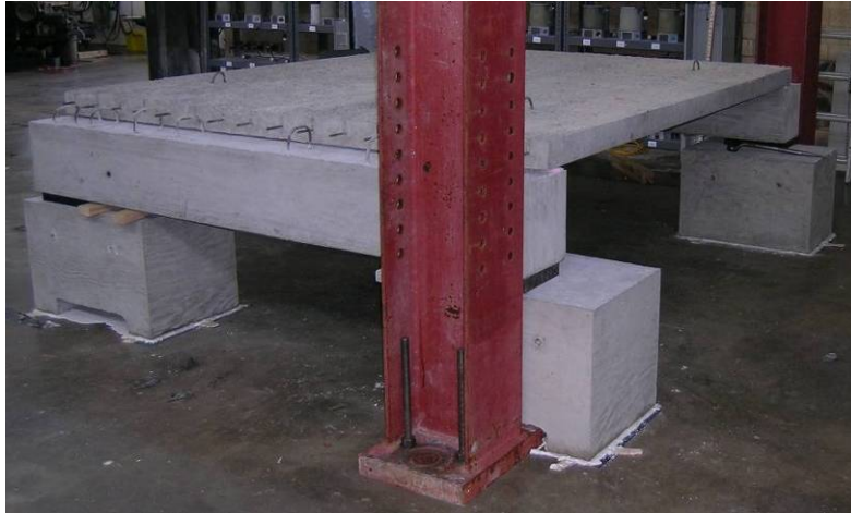
Figure 4.3: Specimen P0P1 After Placing PC Panel
