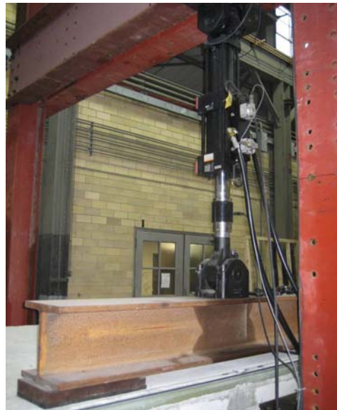
Figure 4.16: Actuator and Spreader Beam for Negative Moment Specimens
